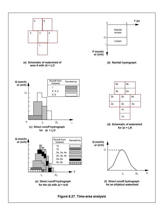
For a rectangular watershed of length L and width W, the direct runoff hydrograph will have the shape of an isosceles triangle, with a peak Ci and a time base of  $2t_c$ . Actual watersheds do not have square edges like the schematic in Figure 6.27a, and they are not rectangular. Instead, they appear more elliptical. In such a case, the hydrograph will have a shape such as that shown in Figure 6.27f.
