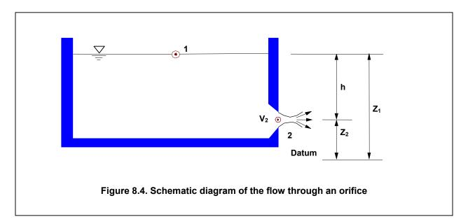
This can be simplified by making the following assumptions: (1) the pressure at both points is atmospheric, therefore  $p_1 = p_2$ ; (2) the surface area of the pool  $A_1$  is very large relative to the area of the orifice  $A_2$ , so from the continuity equation  $V_1$  is essentially zero; and (3)  $z_1 - z_2 = h$ . Thus, Equation 8.7 becomes
