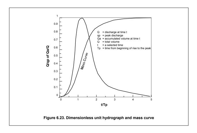
discharge of the curvilinear unit hydrograph. While the time base of the triangular UH is only 8/3 of the time to peak (compared to 5 for the curvilinear UH), the areas under the rising limbs of the two UHs are the same (i.e., 37.5 percent).
