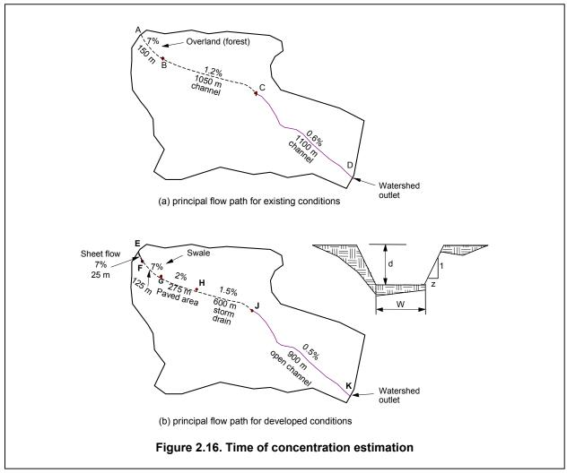
For the section CD, Manning's equation is used. The hydraulic radius is:
