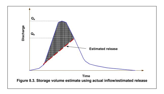
straight line from near the beginning of the rising limb of the inflow hydrograph to the point on the receding limb of inflow hydrograph equal to the maximum release rate. The required volume is represented by the area between the inflow hydrograph and the estimated release rate.
