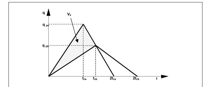
Figure 8.2. Volume of storage (V<sub>s</sub>) determination for the rational formula hydrograph method
