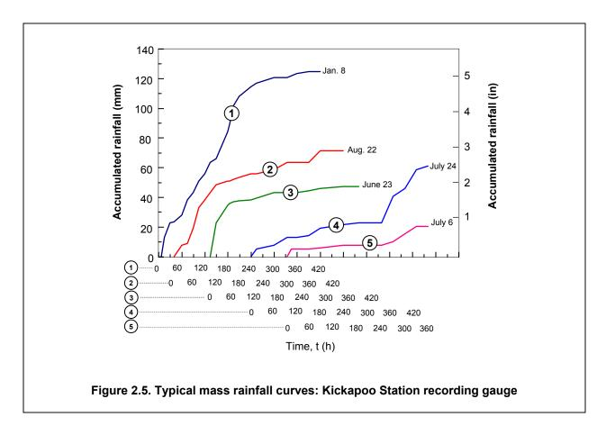
In any given storm, the instantaneous intensity is the slope of the mass rainfall curve at a particular time. For hydrologic analysis, it is desirable to divide the storm into convenient time increments and to determine the average intensity over each of the selected periods. These results are then plotted as rainfall hyetographs, two examples of which are shown in Figure 2.6 for the Kickapoo Station.
