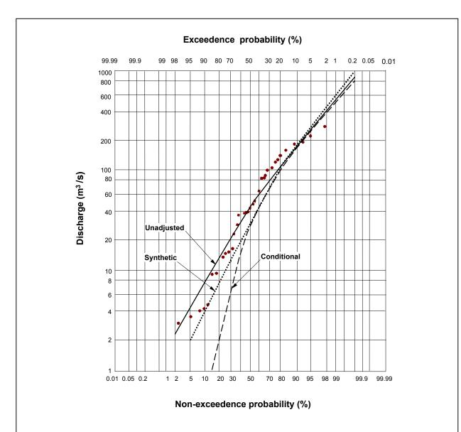
Figure 9.17. Unadjusted, conditional, and synthetic frequency curves, Orestimba Creek, CA
