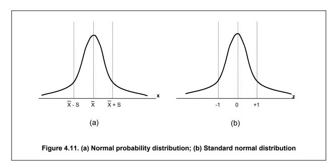
For the normal distribution, the maximum value occurs at the mean. Because of symmetry, half of the flows will be below the mean and half are above. Another characteristic of the normal distribution curve is that 68.3 percent of the events fall between ±1 standard deviation (S), 95 percent of the events fall within ±2S, and 99.7 percent fall within ±3S. In a sample of flows, these percentages will be approximated.
