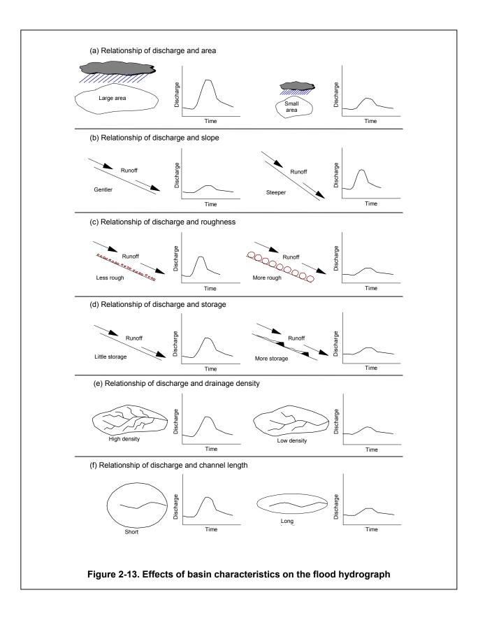
The stage-discharge relationship also can be influenced by storage within a watershed. If the section of a drainage channel is upstream of the storage and within the zone of backwater, the stage for a given discharge will be higher than if the storage were not present. If the section is downstream of the storage, the stage-discharge relationship may or may not be affected, depending upon the presence of channel controls.
