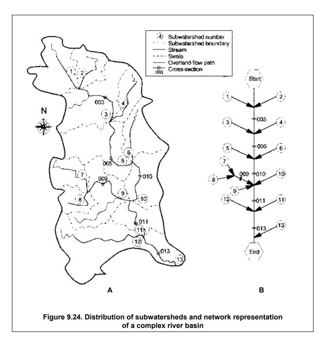
The next step is for the GIS to assist in setting up the data that define the stream network that will control the hydrograph combining and routing. The stream junctions will correspond to the outlet locations of the subwatersheds and represent points where subwatershed hydrographs will be combined before being routed.
