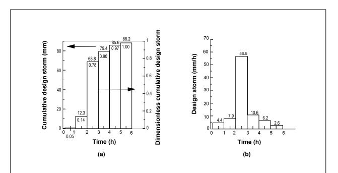
Figure 6.13(SI). 6-hour design storms for Example 6.6(SI): (a) dimensionless cumulative design storm and the cumulative design storm and (b) the design storm
