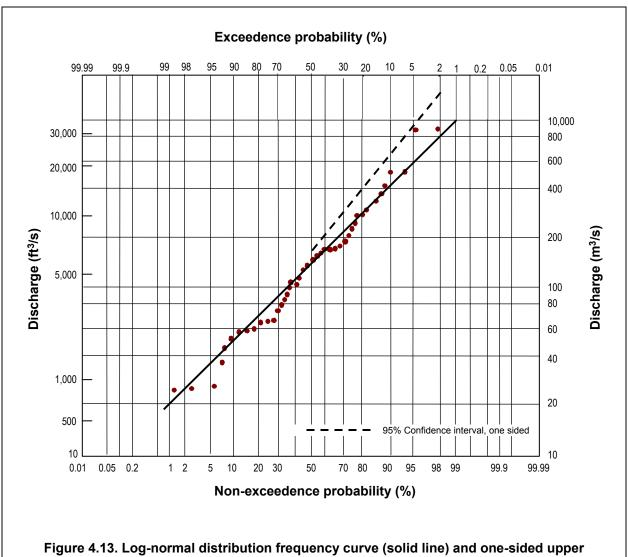
Figure 4.13. Log-normal distribution frequency curve (solid line) and one-sided upper confidence interval (dashed line)
