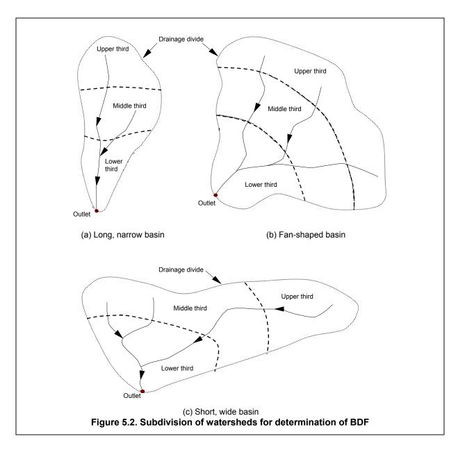
value for a fully developed drainage system would be 12. Conversely, if the drainage system has not been developed, a BDF of 0 would result. Such a condition does not necessarily mean that the basin is unaffected by urbanization. In fact, a basin could be partially urbanized, have some impervious area, and have some improvements to secondary tributaries, and still have an assigned BDF of 0. It will be shown later that such a condition will still frequently cause increases in peak discharges.
