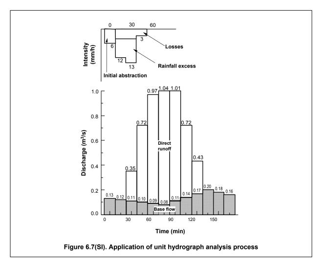
Using the decrease of 0.01 m³/s per 15 minutes produces the base flow rates shown in column 3 of Table 6.1. Since there is a noticeable change of slope on the falling limb of the total runoff hydrograph at a storm time of 135 minutes, this will be used as the inflection point; direct runoff will end at a time of 135 minutes. Thus, the second leg of the base flow function can be represented by a linear segment between storm times of 75 and 135 minutes with a slope of:
