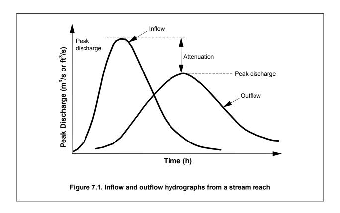
The general equation for channel routing is based on continuity and represents an accounting of all flow within a reach. Mathematically, the continuity of mass can be written in terms of storage as:
