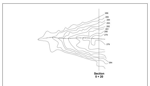
Figure 8.8. Topographic map for deriving stage-storage relationship at site of structure (section 5+20)
