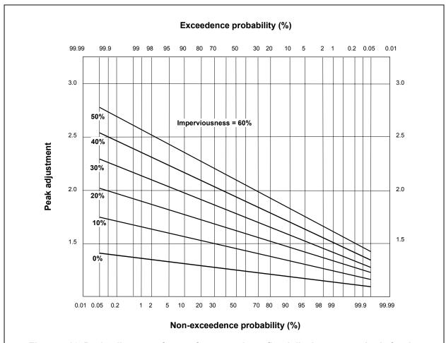
Figure 4.16. Peak adjustment factors for correcting a flood discharge magnitude for the change in imperviousness (from McCuen, 1989)
