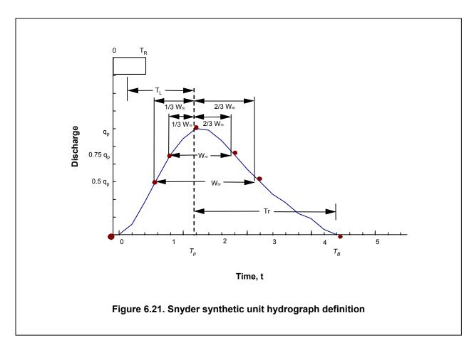
A step-by-step procedure to develop the Snyder unit hydrograph is presented as follows:
