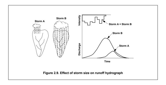
The location of a localized storm in the drainage basin also affects the time distribution of the surface runoff. A storm near the outlet of the watershed will result in the peak flow occurring very quickly and a rapid passage of the flood. If the same storm occurred in a remote part of the basin, the runoff at the outlet due to the storm would be longer and the peak flow lower due to storage in the channel.
