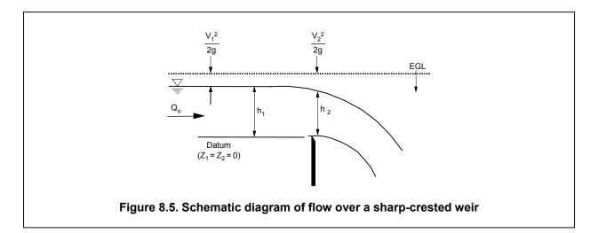
If hydrostatic pressure is assumed at sections 1 and 2, then  $P_i/\gamma = h_i$ . Thus, Bernoulli's equation is:
