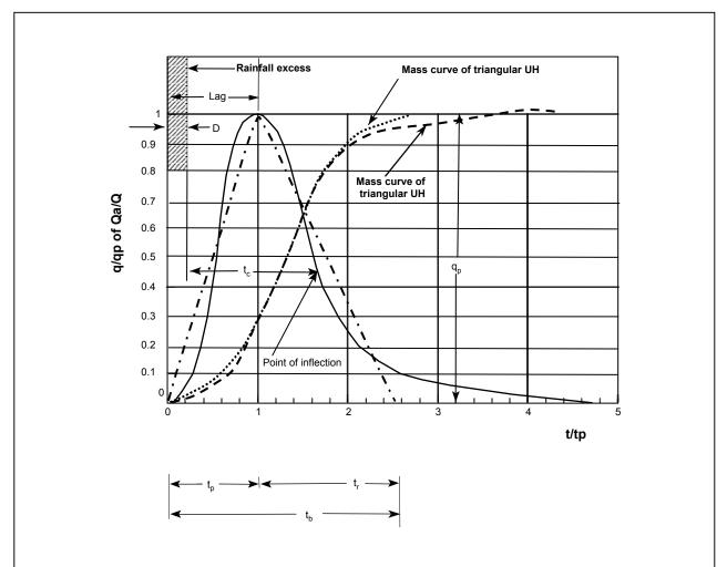
Figure 6.24. Dimensionless curvilinear unit hydrograph and equivalent triangular hydrograph
