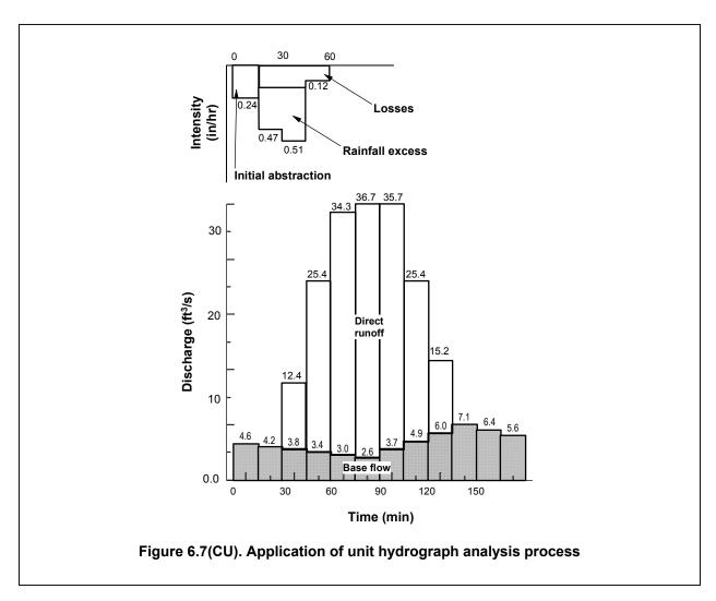
Therefore, the ordinates of the unit hydrograph will be 6.37 times (1/0.157) the ordinates of the direct runoff hydrograph (see column 5 of Table 6.1(CU)). The trapezoidal rule can be used to show that the unit hydrograph represents an average depth of 1 in:
