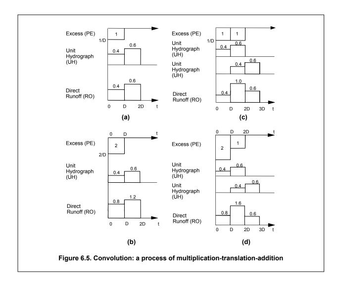
For the case where  $t_{\text{bUH}}$  = 5 and  $t_{\text{bPE}}$  = 3, convolution can be presented by the following equations for computing the direct runoff Q(i) from the rainfall excess P(i) and the unit hydrograph U(i):
