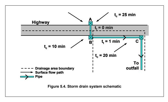
**Example 5.5.** A flooding problem exists along a farm road near Memphis, Tennessee. A low-water crossing is to be replaced by a culvert installation to improve road safety during rainstorms. The drainage area above the crossing is 43.7 ha (108 acres). The return period of the design storm is to be 25 years as determined by local authorities. The engineer must determine the maximum discharge that the culvert must pass for the indicated design storm.
