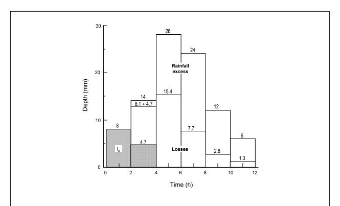
Figure 6.26(SI). Separation of losses and initial abstraction from a design-storm hyetograph using the SCS method.
