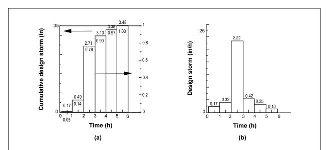
Figure 6.13(CU). 6-hour design storms for Example 6-6(CU): (a) dimensionless cumulative design storm and (b) the design storm
