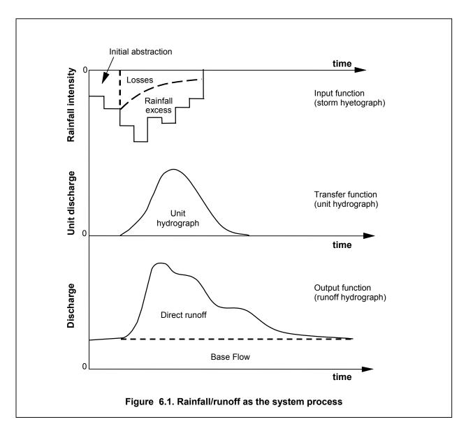
In summary, in the analysis phase, the hyetograph and hydrograph are known and the unit hydrograph is estimated. In the synthesis phase, a hyetograph is used with a unit hydrograph to compute a runoff hydrograph.
