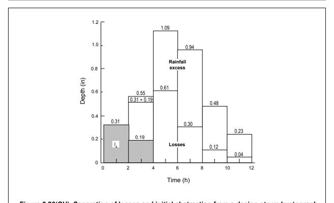
Figure 6.26(CU). Separation of losses and initial abstraction from a design-storm hyetograph using the SCS method.
